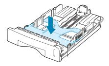
Fan the edges of the paper stack to separate the pages. Then tap the stack on a flat surface to even it up.
